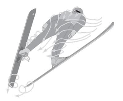
• After flowing around the spread "V" form on the front of the jumper, air then flows over the neck, back and the rear of the legs. A jumper is typically in the air for about four to five seconds. Jumpers generally are no higher than 10-15 feet above the landing hill at any point in the jump. The jumper's downward arc roughly parallels the fall of the slope and landing is usually soft because of the angle of the hill.
